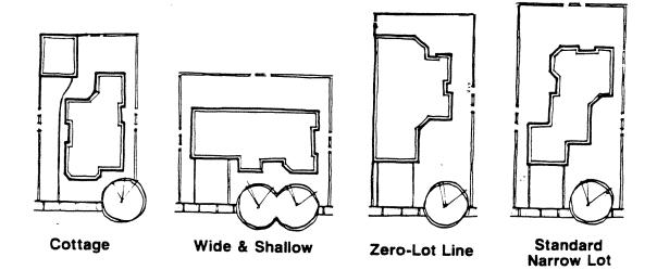
Figure 4.3.1.B. Conceptual Medium Density Residential Building Separation Illustrations
