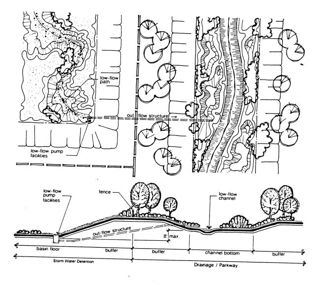
Figure 6.1.2 Detention/Water Quality Basin/Drainage Parkway Interface
