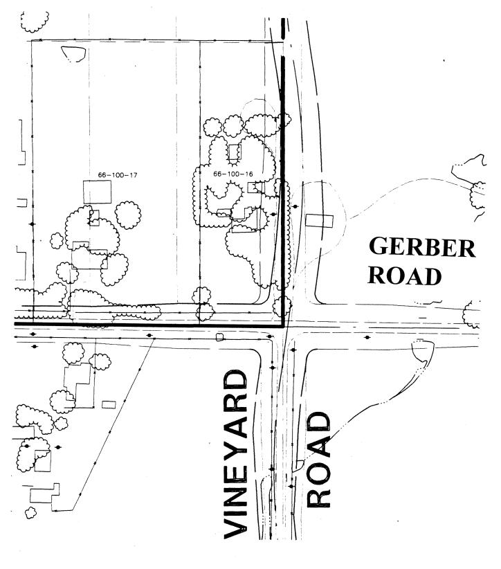
Figure 7.7.2 Conceptual Alignment Plan for the Extension of Vineyard Road
