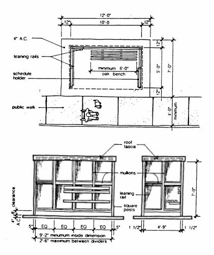
Figure 7.10.6 Bus Shelter Design and Placement
