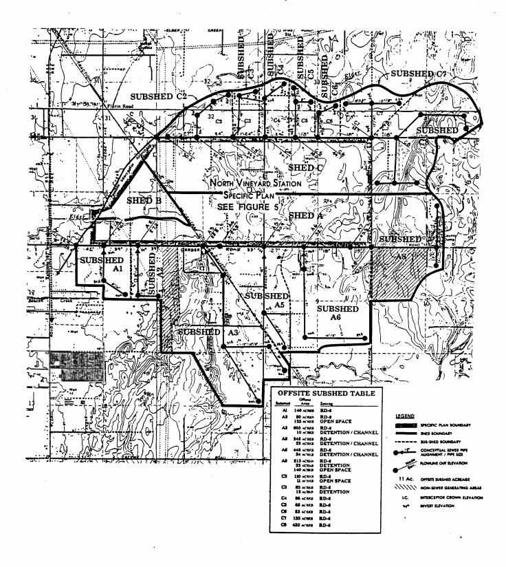
Figure 9.3.3.A. Off-site Sanitary Sewer Facilities .
