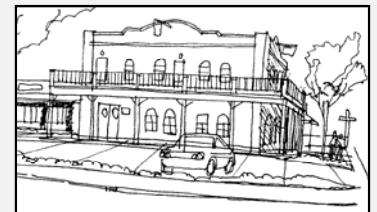
Simple parapet (not ornate)
